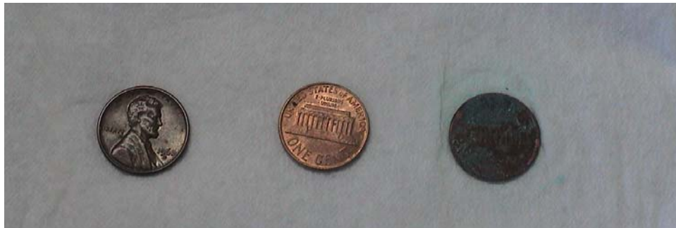
(L to R) dirty penny, cleaned penny, penny which is oxidized with prolong exposure to vinegar solution.
